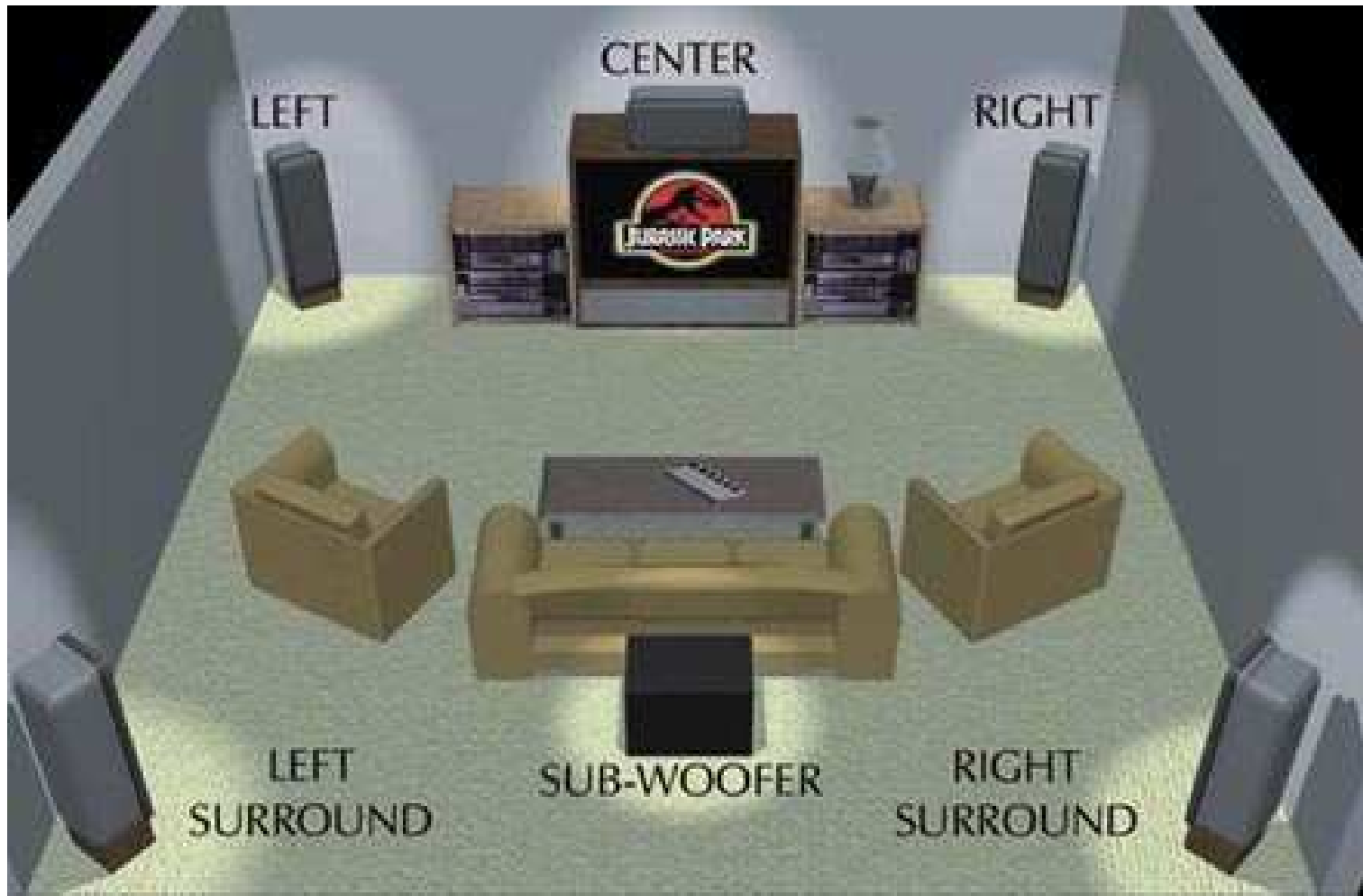
Figure 1: Example Surround Sound Layout [5]
